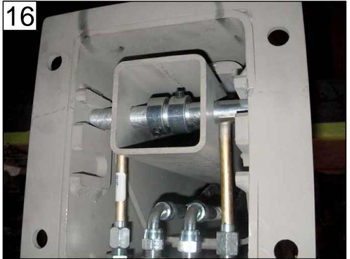
PUSH SHAFT INTO TOP SLOT OF CROSSTUBE
