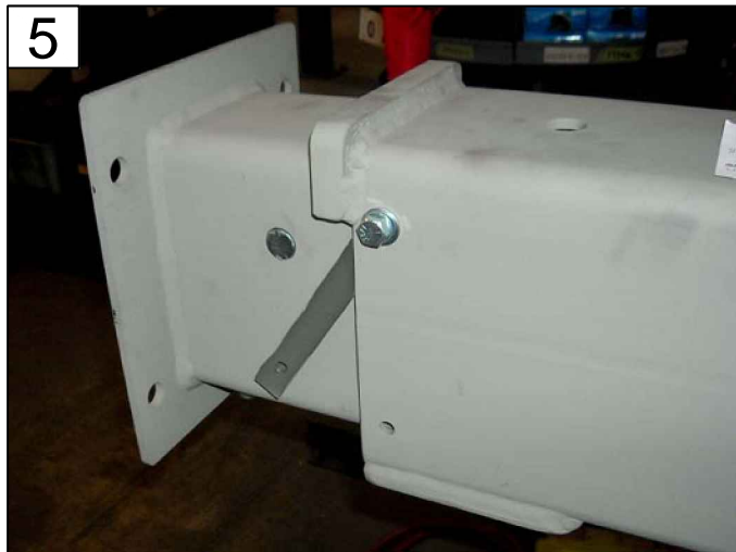
FASTEN 25065 NUT BAR RETAINERS IN CROSSTUBE PAGE 15 - ITEMS 2, 7, 8, & 9
