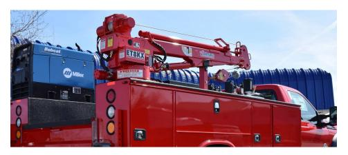
The Venturo ET8KX is a 8,000 ft-lb electric-hydraulic service crane with a 3,200 lb lifting capacity featuring 12V DC electric winch, hydraulic rotation,, hydraulic boom elevation with a hydraulic extension and secondary manual extension. The ET8KX also has optional proportional controls which allow the operator additional control over speeds of the hydraulic functions.
