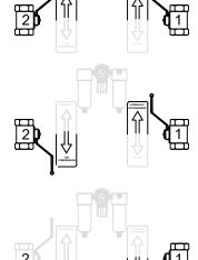
FOR STABILIZER OPERATION **DIVERTER HANDLE #1 UP DIVERTER HANDLE #2 UP**
