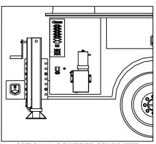
OPTIONAL: **POWERED STABILIZER**POWER UNIT AND CONTROLS
