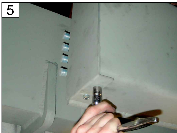
5 FASTEN END CAP COVERS FLUSH AGAINST CROSSTUBES PAGE 17 - ITEMS 5, 12, 13
