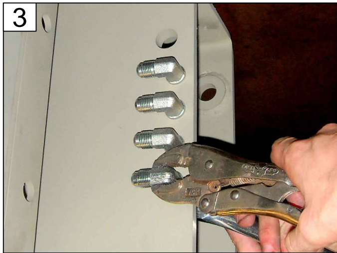
3 FASTEN BULKHEAD FITTINGS, POINTING CURB-SIDE PAGE 17 - ITEM 9
