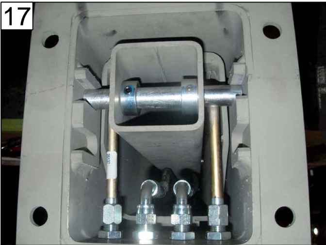
WITH CYLINDER HOUSING CENTERED LOCTITE & FASTEN COLLARS FLUSH
