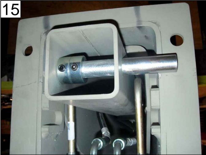
INSERT SHAFT & COLLARS INTO CYLINDER HOUSING
