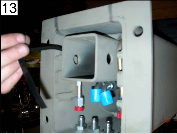
UNTIE PULLOUT CYLINDER HOUSING & PLUMBING
