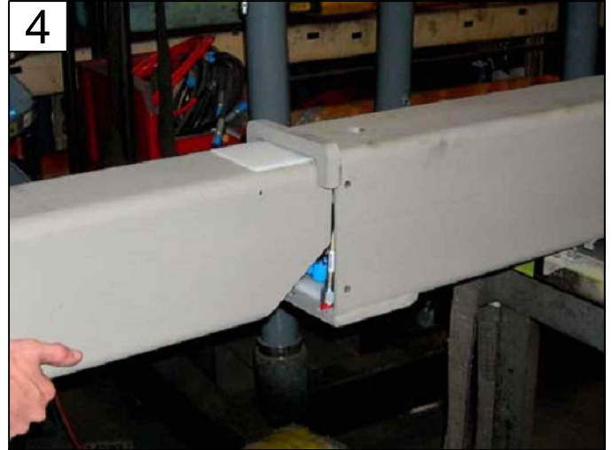
SLIDE PULLOUT INTO CROSSTUBE
