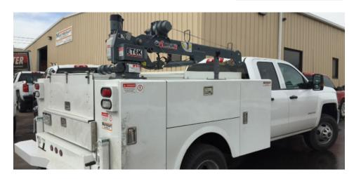
The ET6K service crane is a light-weight, cost-effective choice for a variety of industries and general service applications on any truck with a GVWR of 8,000 lbs or less. The ET6K features 2,000 lbs of maximum capacity and a 6,000 ft-lb crane rating.
