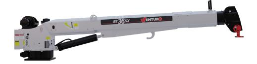
The Venturo ET36KX is a 36,000 ft-lb electric-hydraulic service crane with a 6,000 lb maximum capacity at 6 ft. This larger crane gives operators the distance and strength they need for heavier loads at a short distance. This electric crane features full-hydraulic boom extension out to 20 ft.
