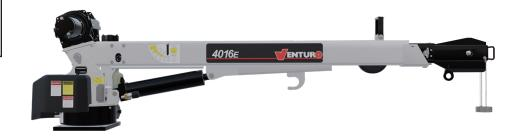
The Venturo 4016E is a 16,000 ft-lb electric-hydraulic service crane with a 4,000 lb maximum capacity. This crane allows operators a crane application without the need for a heavy crane service body. A reinforced crane compartment on a standard utility body provides operators the strength they need on a standard service truck.
