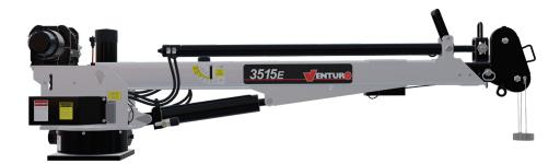
The Venturo 3515E service crane is a versatile application that is neither too large or small for a majority of lifting jobs. This crane has been utilized heavily in municipal/ public works lifting anything from service equipment to fire hydrants throughout the United States. With a 12,000 ft-lb crane rating and a 3,500 lb maximum capacity, the 3515E can be installed on trucks with a minimum 8,800 lbs GVWR.
